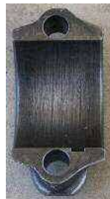
Damaged conrod cap
