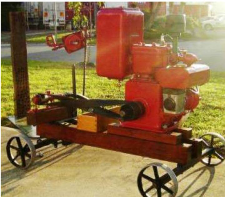
Gane engine with attached Post drill
