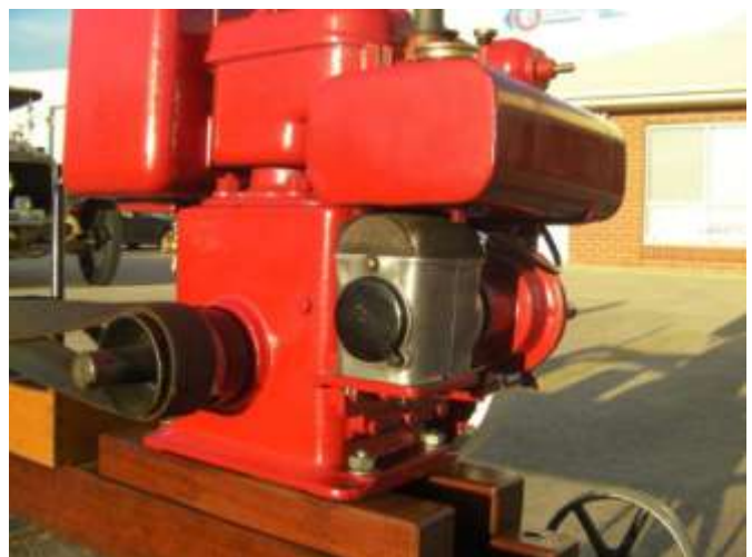
Gane engine showing the vertical mounted magneto
