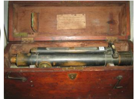
Dumpy Level, note label on instrument and box
