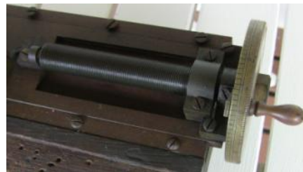
Inscribing Tool (detail of fine pitched advancing screw)
