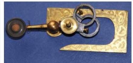
Microscope Accessory (specimens held in the rings can be turned over) owned by Dick Turpin
