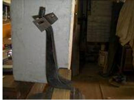
One morning I went down to the shed and studied the bracket. It is basically a "U" shape but tapering in its length and has 3 bends on each plane or side. I thought if I get the empty cereal box left from breakfast and trace each face onto the cardboard, I may be able to cut these out of 3mm sheet steel and weld them together. I did this on the three faces, marking the centre line of each bend and adhered these to a piece of 3mm flat steel with spray contact.
