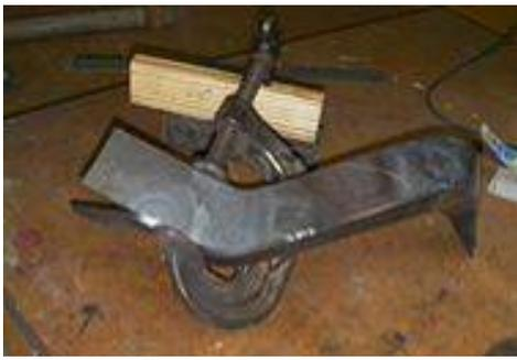
I then completed all welding and finished off all welds and round over edge to make it look like it has been pressed.
