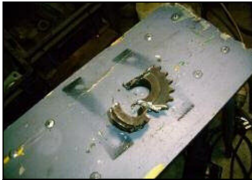
Remains of the sprocket
