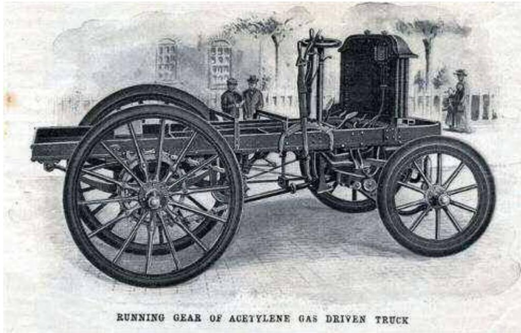
RUNNING GEAR OF ACETYLENE GAS DRIVEN TRUCK
